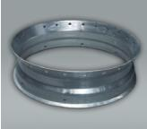
**12 GA. HOPPER COLLAR** The hopper collar is a critical component of the Bulk Feed Tank. AP's 6', 7', 9' and 12' bulk feed tanks utilize a 12 gauge hopper collar, producing a part that is 30% stronger than the industry standard 14 gauge collar.
