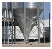
**60° & 67° HOPPER SLOPES** Available in 60° and 67° slopes in either a 16" or 22" hopper opening, AP hopper panels are die-formed with rounded corners and down-turned sealing edges for safety and a weathertight fit. Assembly with rounded, truss-head bolts reduces content bridging.
